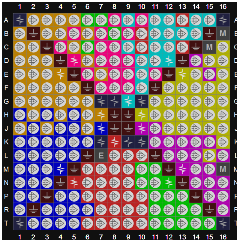
Figure 3-2 View of GW2A-18 PG256 Pins Distribution (Top View)
